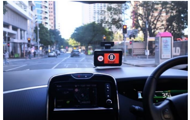
Figure 2: Example of ARLW message shown before a red light (Image source: Queensland Government).
