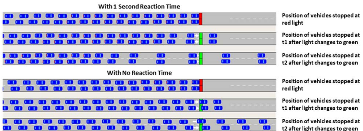
Figure 2 An illustration that shorter reaction time can increase the throughput at a traffic light
