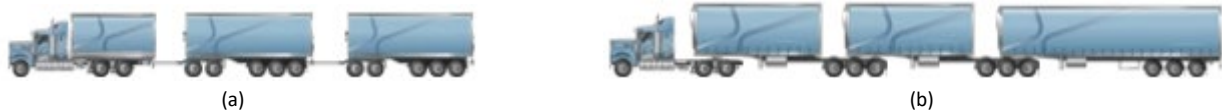
Figure 4 (a) Trailers connected with draw bar (also known as dog trailer), (b) Trailers connected on turn table.
