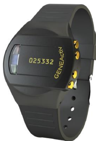
Figure 7: Wrist-worn accelerometer-based device, GENEActiv
