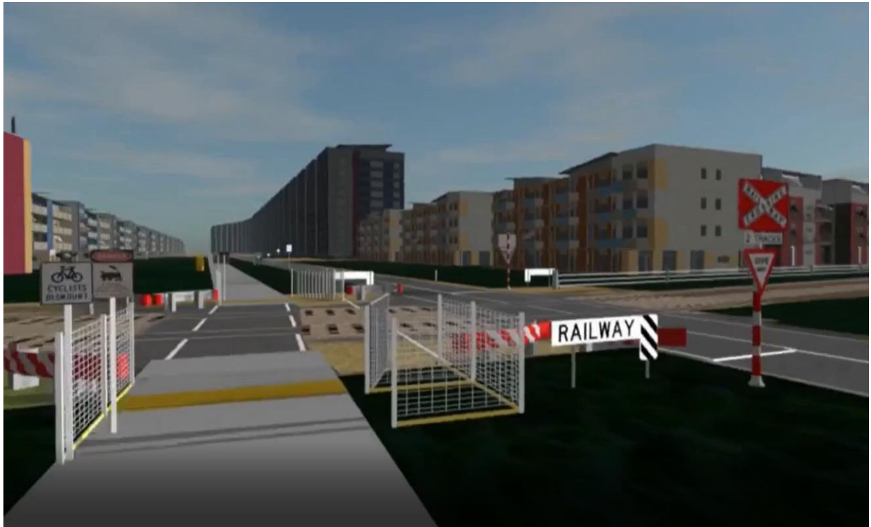
Figure 3: Passive control level crossing
