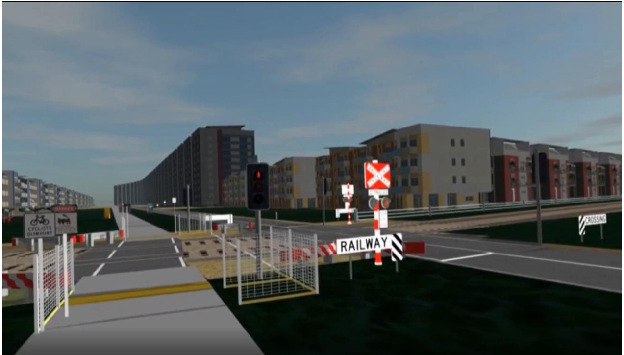
Figure 4: Active control level crossing
