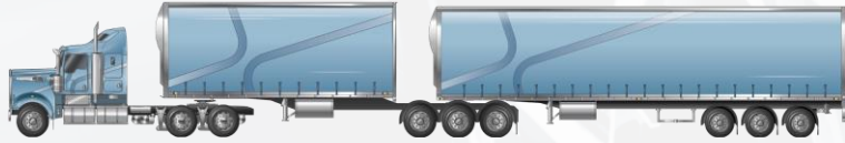
26m Conventional B-Double (General Mass Limits) 62.5t Gross combination mass 37.28t Payload
