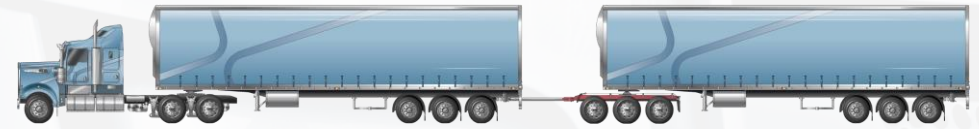
30m PBS A-Double (Higher Mass Limits) 85t Gross combination mass 55.07t Payload
