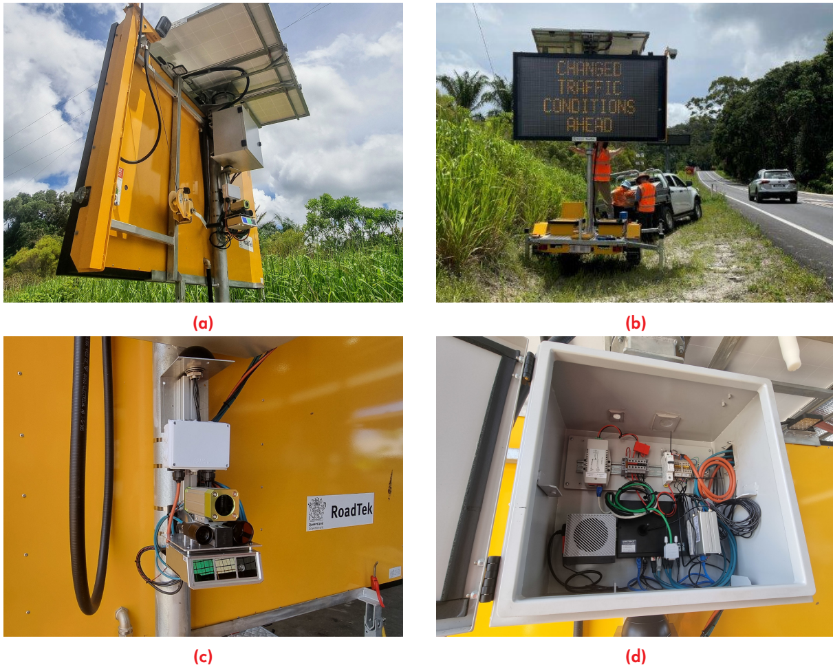
Figure 6.1.: Installation of the animal detection system onto the VMS trailer and its deployment in the field are shown. (a) shows the VMS trailer in the field with the detection system installed. In (b), the VMS trailer is being set up in the field. (c) takes a closer look at the sensor head of the detection system installed onto the pole of the VMS trailer. Its components, from top to bottom, include: a black cap housing WiFi, GPS, and 4G antennas for communication; a white electrical junction box; an aluminium enclosure for the thermal camera; two RGB cameras (the left being the medium-angle camera and the right, the telephoto camera); and the solid-state LiDAR. (d) shows the edge computing and networking devices, as well as cabling in the control box. From left to right: the NVIDIA Orin computing unit; the QNAP network switch; and the Teltonika router.
