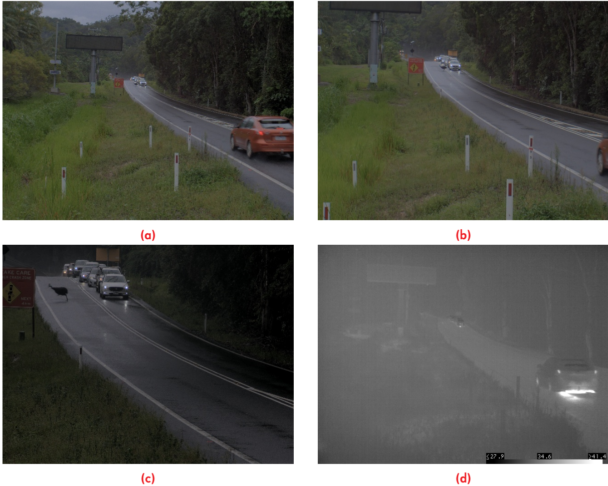
Figure 6.4.: An example of a cassowary crossing case at a distance of 180 metres from Location A. (c) shows the cassowary on the road in the telephoto camera image. (a), (b), and (d) show the same cassowary in medium-angle, digital-zoomed, and thermal images, respectively. As the figures illustrate, the cassowary appears too small to be detectable in (a), (b), and (d).
