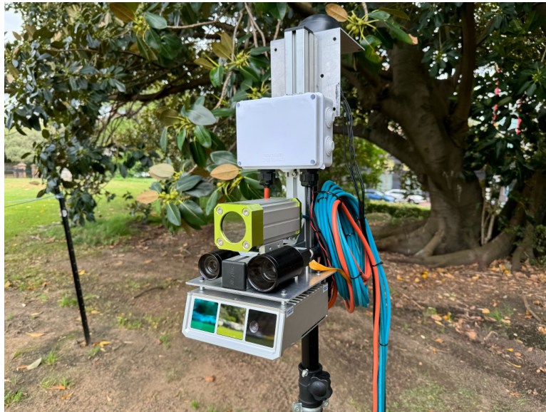
Figure 3.1.: The sensor head developed for animal detection. Its components, from top to bottom, include: a black cap housing WiFi, GPS, and 4G antennas for communication; a white electrical junction box; an aluminium enclosure for the thermal camera; two RGB cameras (the left being the medium-angle camera and the right, the telephoto camera); and the solid-state LiDAR. In the picture, the sensor head is shown temporarily mounted on a tripod for outdoor testing.
