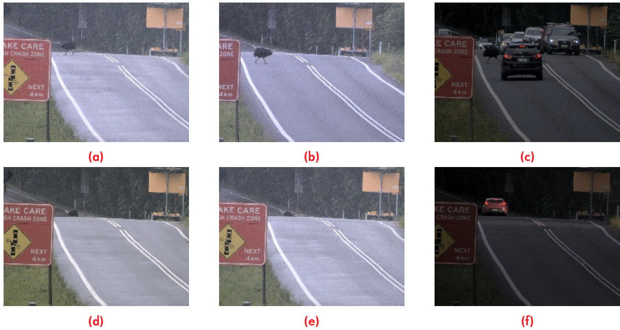
Figure 6.11.: Sensor occlusion examples at Location A. (a) - (f) illustrate cases with different severity levels of sensor occlusion caused by environmental and traffic factors, such as the red warning signage, the hilly terrain, and vehicles. When the cassowary is crossing from left to right, the occlusion caused by the warning signage eliminates the advantage of detecting the animal early on, before it crosses the road. As (d) and (e) show, the partial occlusion caused by the hilly terrain for distant cassowaries presents challenges for the cassowary detector. Lastly, vehicles on the road also cause temporary occlusion for the cassowaries, as (c) and (f) illustrate. In (f), a cassowary was heavily occluded by both the signage and the red car.
