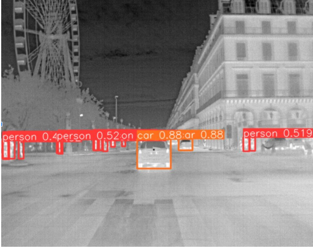
Figure 3.13.: Results of applying domain adaptation to thermal images. By employing transfer learning, the detection model is fine-tuned to operate effectively within the thermal image domain.
