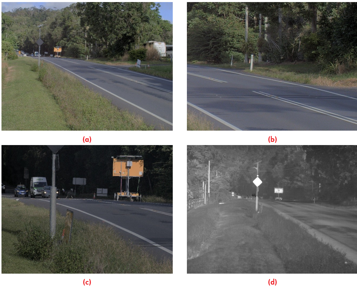
Figure 6.6.: Another example of cassowary crossing case with a distance of 135 metres from the Location B. (a), (c), and (d) show the same cassowary in medium-angle, telephoto, and thermal images, respectively. (b) shows the view from the digital-zoomed image. As the figures illustrate, the cassowary appears a good size to be detectable by YOLOv8 in the telephoto image.
