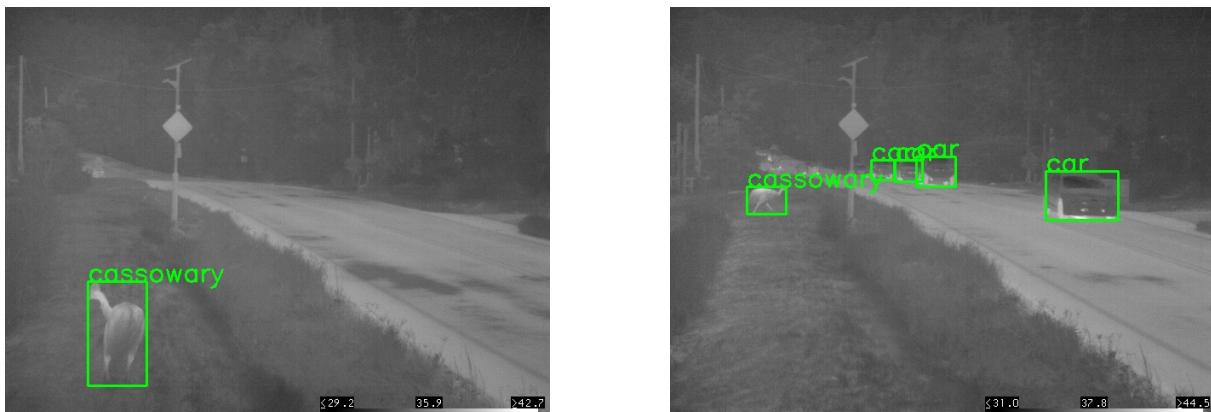
Figure 6.10.: The images illustrate the effectiveness of our pipeline on thermal imagery. Initially pre-trained on RGB images, the model has successfully adapted to process thermal images.
