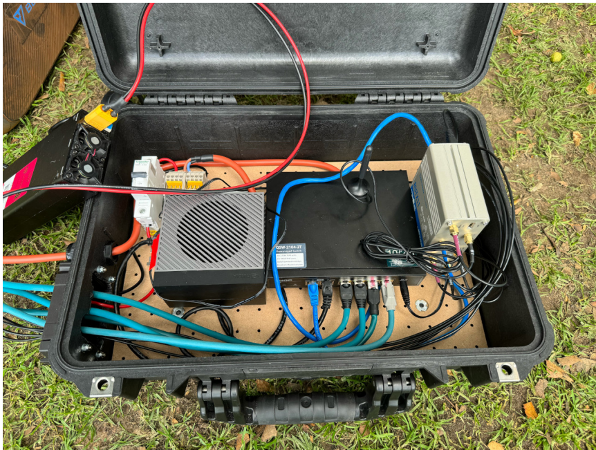
Figure 3.2.: The networking and edge computing for the developed system. From left to right: a white electrical circuit breaker; the NVIDIA Orin computing unit; the QNAP network switch; and the Teltonika router. These devices were temporarily housed in a Pelican protector case for outdoor testing, as shown in the picture.
