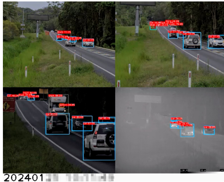
Figure 6.3.: A screenshot of the H.265 video recording shows example RGB and thermal camera images from Location A. Top left: RGB image from the medium-angle camera; Top right: digitally zoomed RGB image from the medium-angle camera; Bottom left: RGB image from the telephoto camera; Bottom right: image from the thermal camera. The timestamp of these images is shown at the bottom. Each image also has the overlay of bounding boxes of detected objects generated by its corresponding YOLOv8 detection model.
