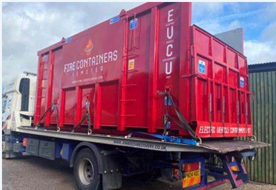
Figure 14: Fire-resistant container for transporting damaged EVs by SEDA-Umwelttechnik GmbH [80]
