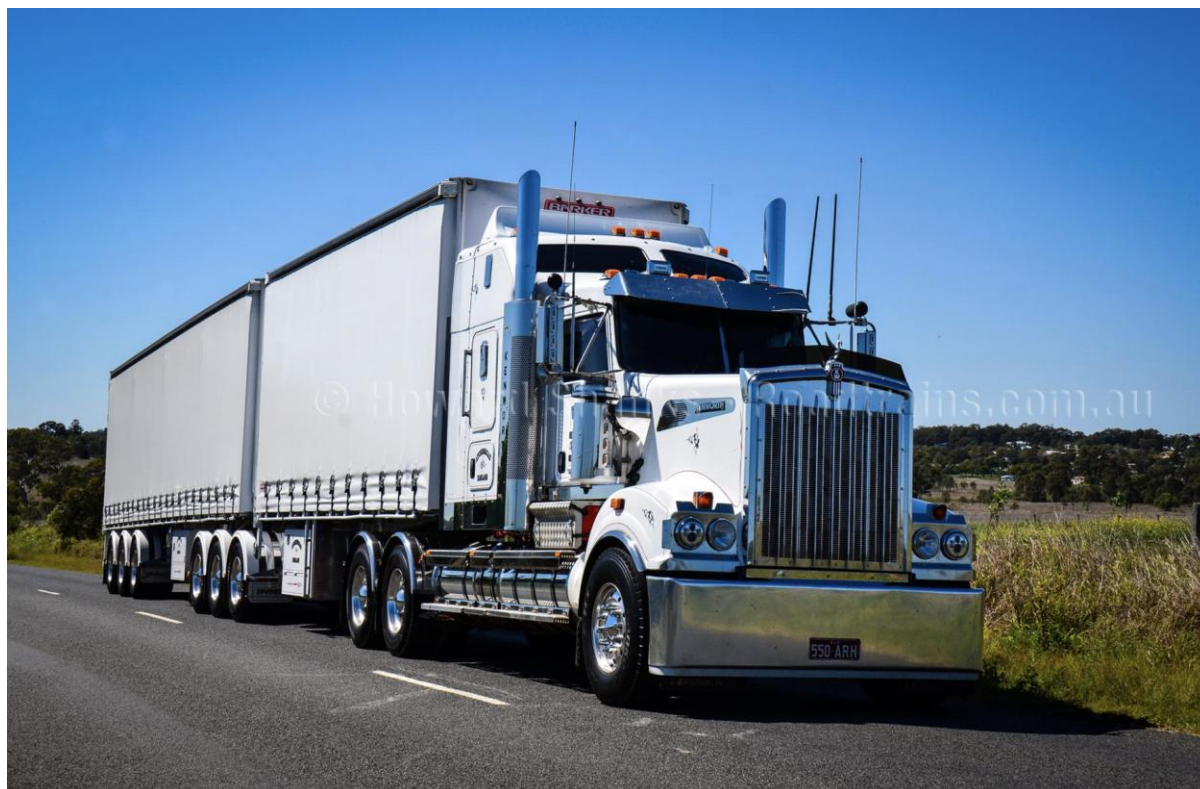
Figure 2-2 A 27 metre B-Double prime mover and road-train
