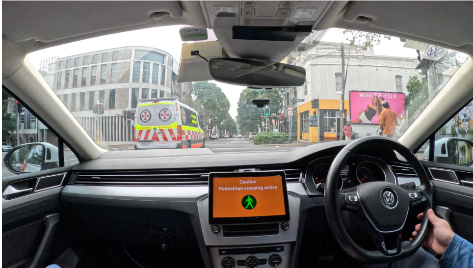
Figure 6.11: Driver alerting when approaching active pedestrian crossing
