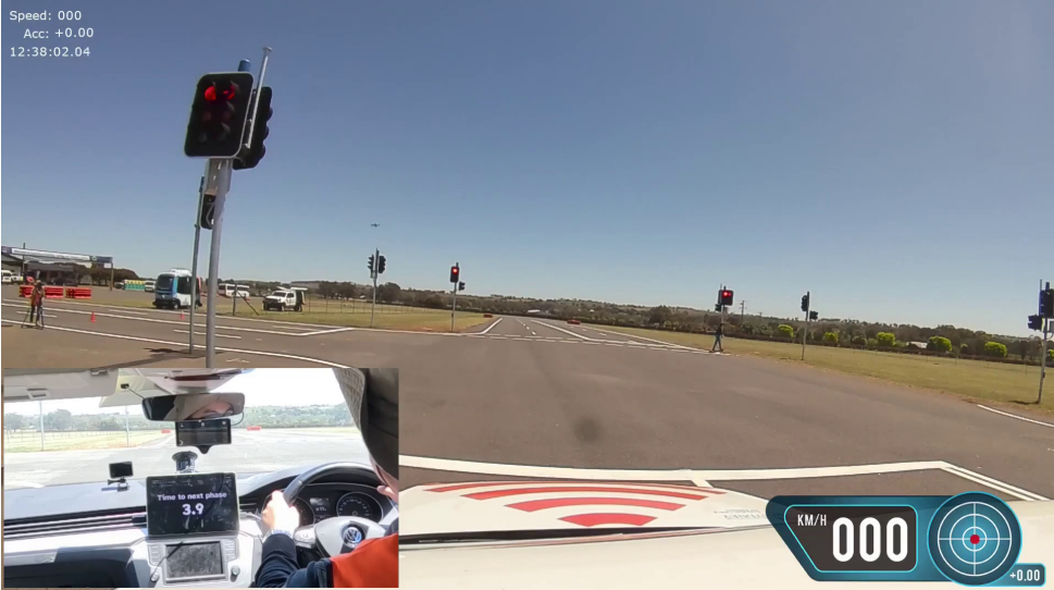
Figure 6.15: In-cabin time to green information was shown to the driver in FMTRC demonstration
