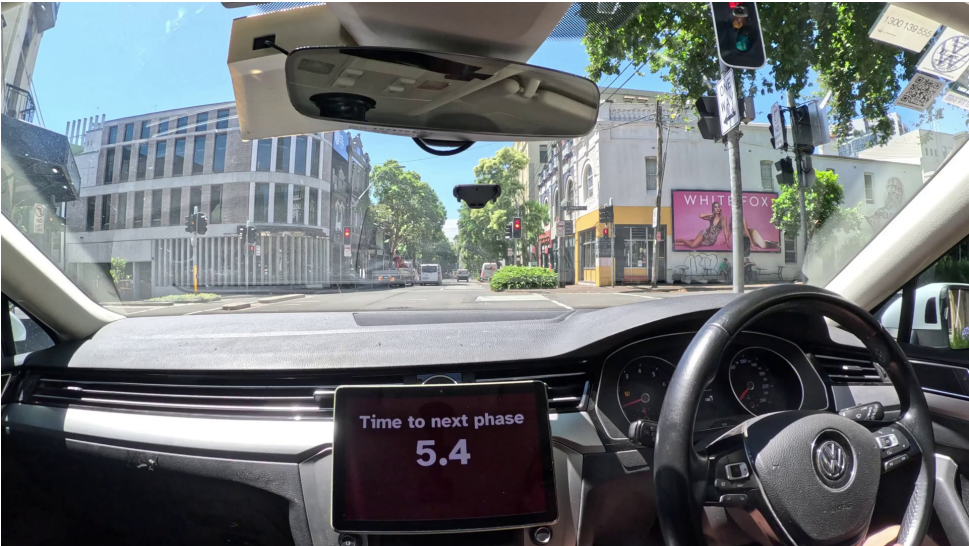
Figure 6.16: In-cabin time to green information was displayed to the driver in live traffic demonstration
