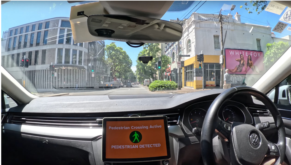
Figure 6.13: Driver alerting when approaching active pedestrian crossing with a pedestrian in the pedestrian crossing
