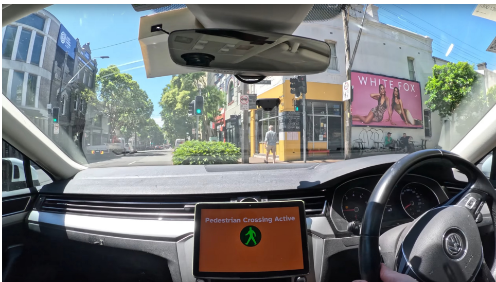
Figure 6.14: Driver alerting when approaching active pedestrian crossing, but the pedestrian has exited the pedestrian crossing
