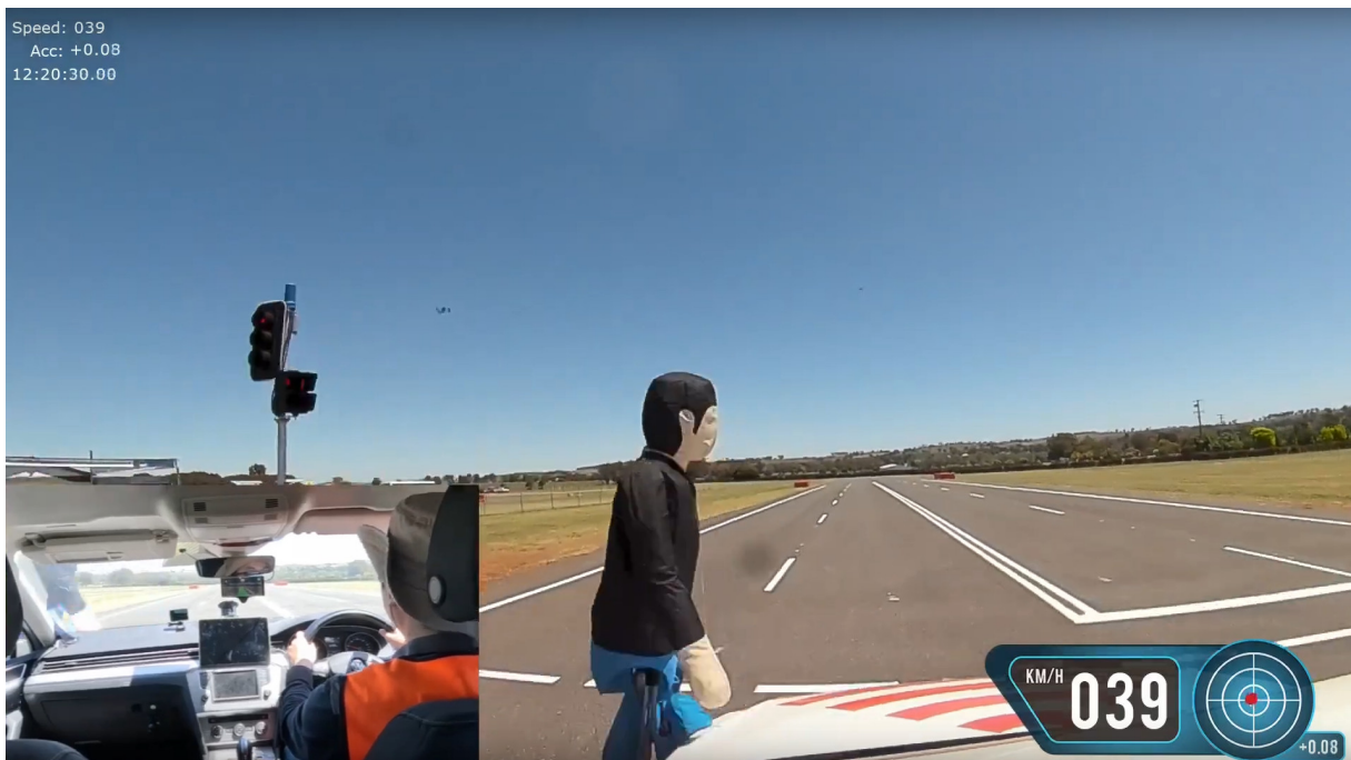
Figure 5.2: A lack of RLVW results in a driver striking a pedestrian after violating a red light
