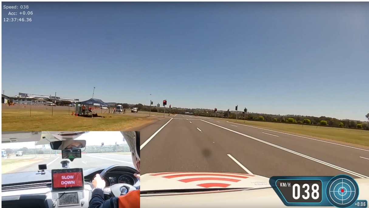
Figure 5.1: An in-cabin RLVW enables the driver of a CV to come to a safe stop
