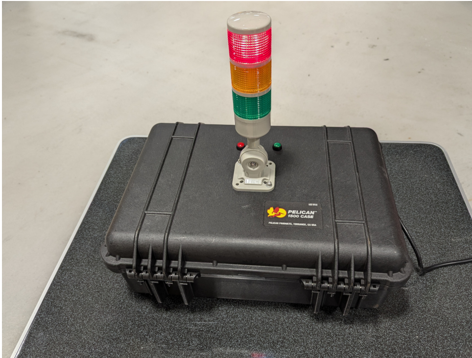
Figure 4.3: DSRC-enabled mock traffic lights
