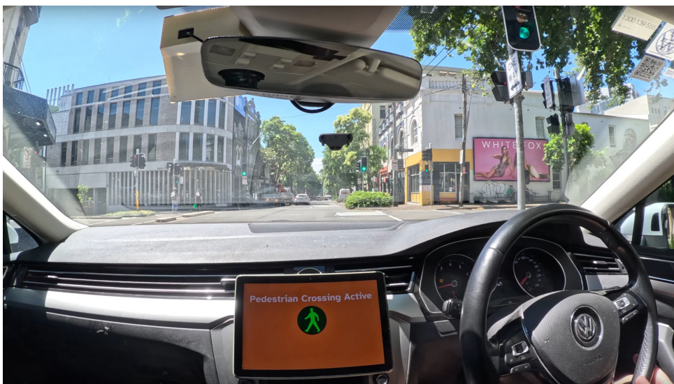
Figure 6.12: Driver alerting when approaching active pedestrian crossing, but no pedestrian in the pedestrian crossing
