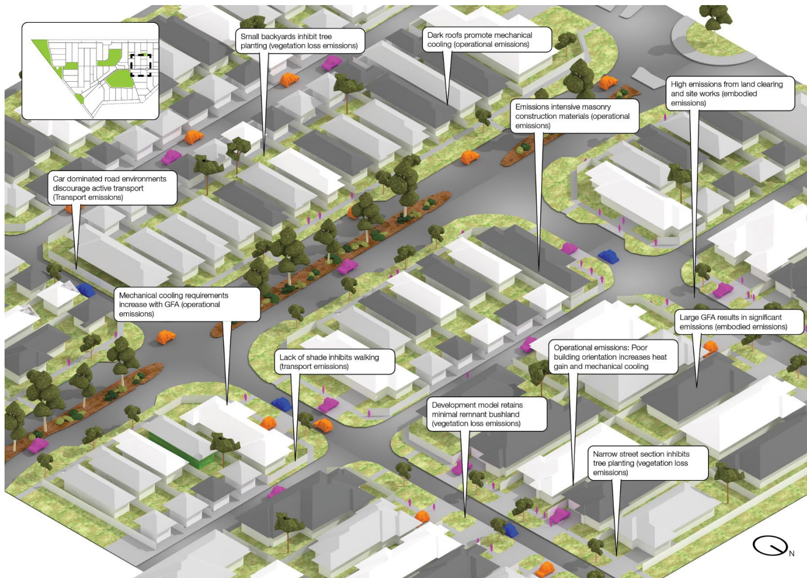
Figure 16: Jindalee study site 2- existing.
