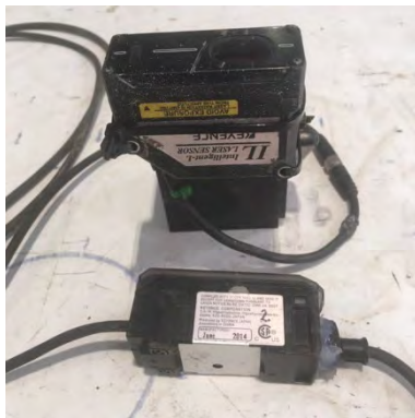
(a) Laser displacement sensor
