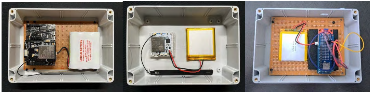
Figure 3.1: From left to right, Libelium Waspote, RAKwireless WisTrio RAK5010 and Arduino MKR NB1500.
