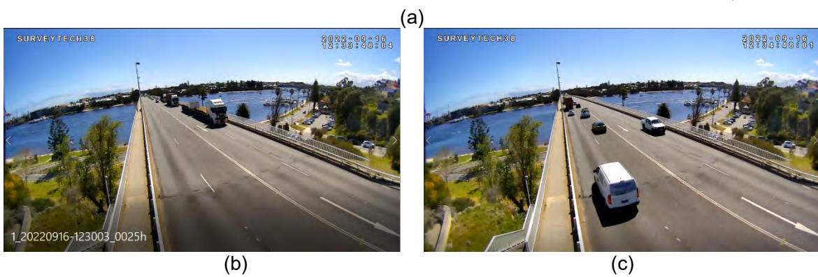
Figure 4.12: (a) bridge dynamic displacement between 12:33-12:37 Sep 16, 2022; (b) traffic pattern at 12:33:48 Sep 2022: heavy vehicles mainly distributed on the Fremantle-Perth city direction traffic line; (c) traffic pattern at 12:34:48 Sep 16 2022: heavy vehicles mainly distributed on the Perth city-Fremantle direction traffic line.
