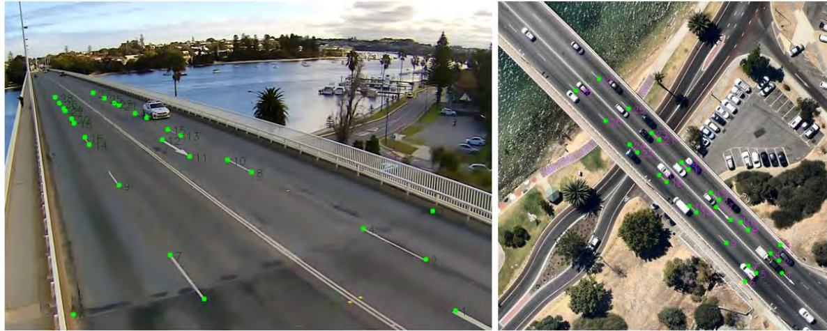
Figure 2 – Key points used to estimate the homographic transformation
