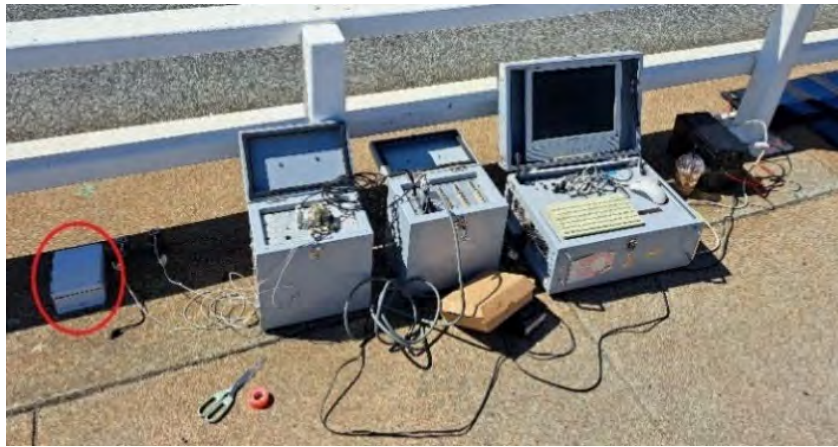
Figure 4.5: Sensors placed roadside at Stirling Bridge. Highlighted in red is the IoT prototype.
