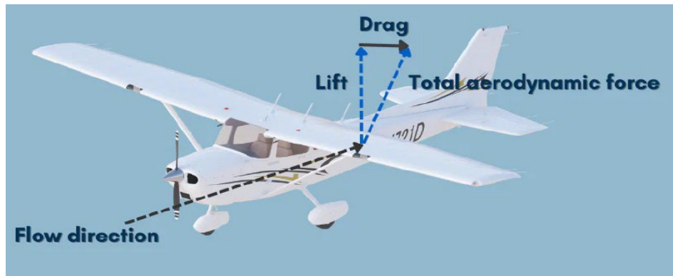
Figure 3.15: Simple schematic representation of lift induced drag
